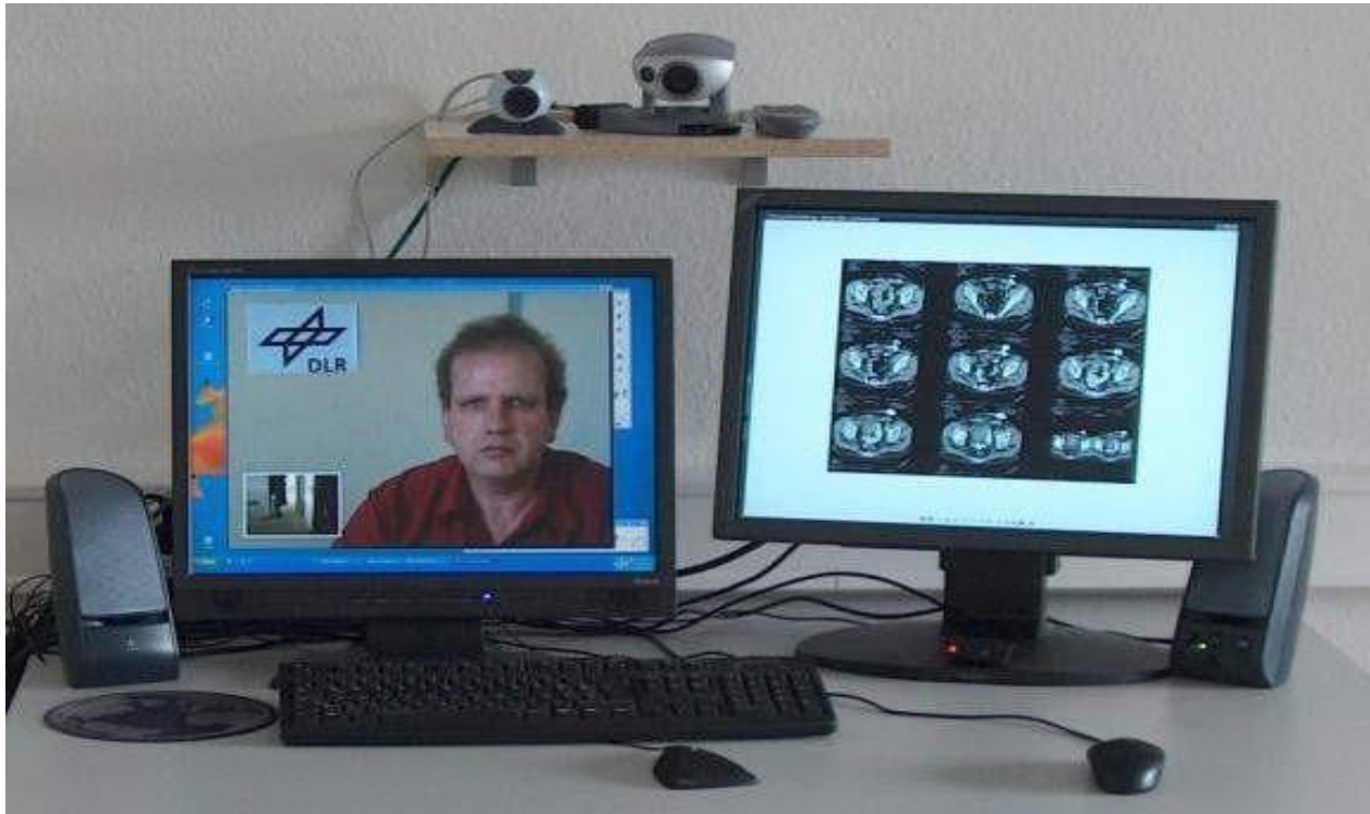
Figure 5: Teleradiology system with video conferencing component for teleconsultation 14
