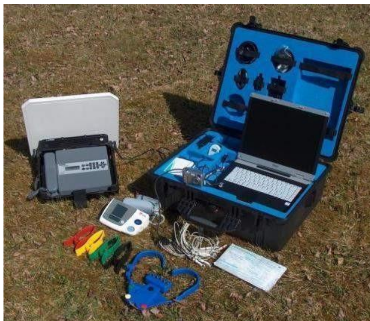
Figure 4: Satellite-based transportable telemedicine system 13
